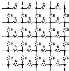
Between every pair of adjacent nodes is a resistance  $R$ . The grid extends to infinity in all directions. Determine the effective resistance between any two adjacent nodes in the lattice.
